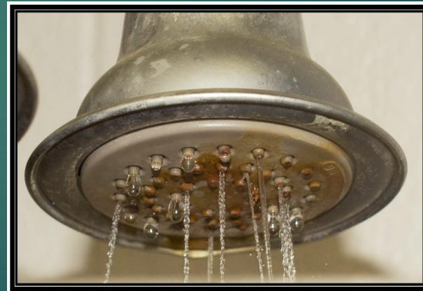
Figure 6-10D. Showerhead 10 on seventh day of testing with hard well water (28 grains per gallon) showing spray pattern. Battelle testing for Water Quality Association. May 1, 2009
