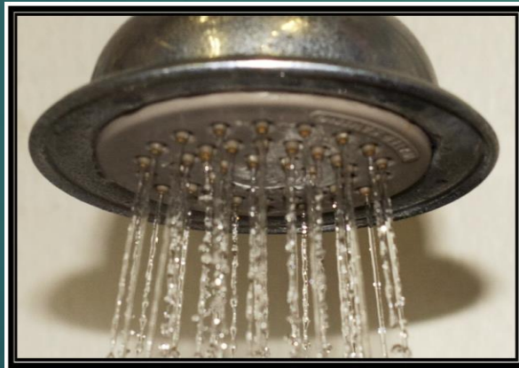
Figure 6-5D. Showerhead 5 on seventh day of testing with soft well water (<1 grain per gallon) showing spray pattern. Battelle testing for Water Quality Association. May 1, 2009
