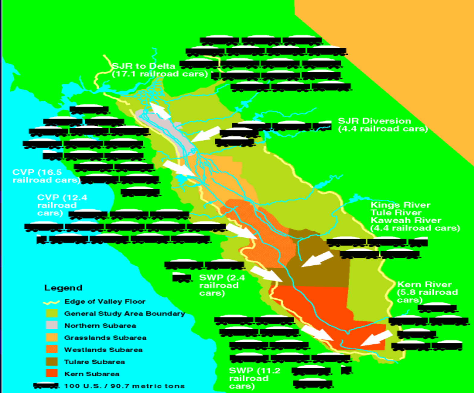
Surface Water Salt Inflow/Outflow (railroad cars per day) Westside of San Joaquin Valley
